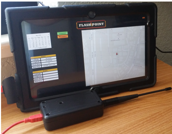
Fig. 48: Flashpoint V 0.50 Receiver Hardware and User Interface [7]
